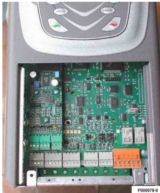
Fig. 64: Encoder board fastened to its slot
